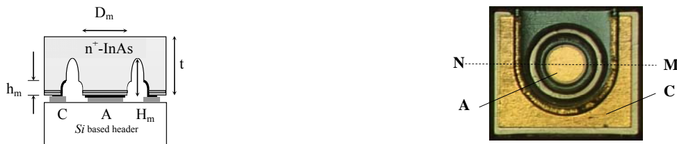
Fig. 2 Schematic of the InAs deep mesa “flip-chip” LED grown onto n^+ -InAs and mounted onto Si header (cross section in the N-M direction) (at the left) and photo of the unmounted chip with contacts (at the right). D_m - is the mesa diameter, h_m - is the distance from the p-InAsSbP surface to the deepest cathode areas, (“depth of the cathode”), H_m - is the total depth/height of the internal reflector, t - is the total p-InAsSbP/n-InAs/ n^+ -InAs structure thickness, A- is the anode, C- is the cathode.
