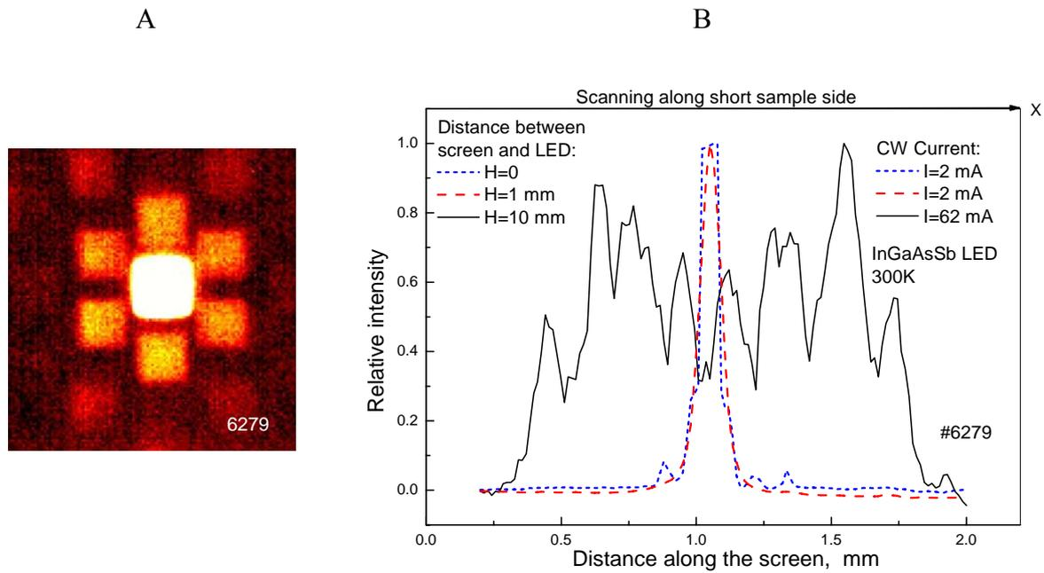
Fig. 3. A – IR image of PC LED emitting surface at forward bias; B - radiation pattern directly over outcoupling surface (“near-field”) and over the screen placed at a distance of 1 and 10 mm from the chip surface. Field of view; 400x400  $\mu\text{m}$  (A) and 2x2 mm (B). See axis X in Fig.1 as well.
