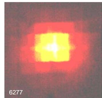
“duplicates” (Fig.3) arranged in a hexagonal geometry. The difference between IR images in Fig.2 and Fig.3 arises from the difference in lateral dimensions. As Fig.2 presents device with rather “big” mesa lateral dimensions (130x130 μm) the overlapping of diffraction images is taking place. Quite small element dimensions of the second LED (70x70 μm) prevents above overlapping and fair good resolution of the “orders” is taking place.
