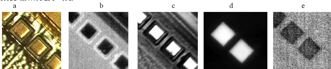
**Fig.3** Photo (a) and IR images (b, c, d, e) of a diode array where dark color corresponds to low emissivity/apparent temperature  $T_a$  while white color corresponds to high emissivity/apparent temperature  $T_a$ . a, b, c – measurements from the epi-side, d, e – measurements from the substrate side ( $n^+$ -InAs) with external lightening  $\lambda = 2.9 \mu\text{m}$  (c) and bias (d, e). d- forward bias is applied to two array elements, e – reverse bias is applied to three array elements.
