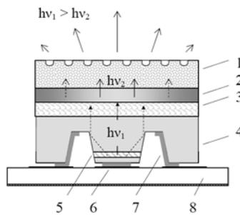
**Fig. 1** Scheme of an optically pumped LED with PC (bottom) where 1-  $n^+$ -InAs substrate with periodic structure, 2-  $n^0$ -InAs layer, 3- optical glue, 4 -GaAs LED in which 5- active area, 6- anode, 7- cathode, 8- Si submount. Upper part: SEM image of  $n^+$ -InAs outcoupling surface. Horizontal white line corresponds to a distance of 3  $\mu\text{m}$ .
