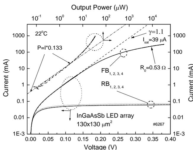
**Fig.4** Typical I-V (left and low scales) and L-I (right and upper scales) characteristics of array elements #1, #2, #3, #4. Dotted line presents the function of the form  $I = 0.039(\exp(U/\gamma kT) - 1)$ ,  $\gamma = 1.1$ , where  $U$  – bias voltage,  $I$  – current
