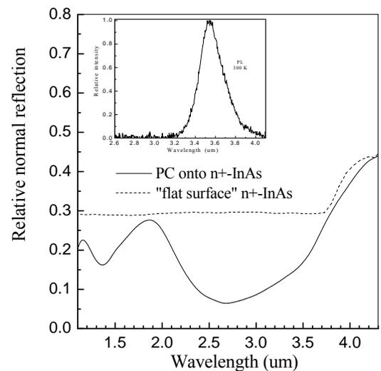
**Fig. 2** Reflection coefficients for a normal rays when measured on plane samples from 350  $\mu\text{m}$  thick  $n$ -InAs (dotted line) and 500  $\mu\text{m}$  thick  $n^0$ -InAs/ $n^+$ -InAs structures with PC onto  $n^+$ -InAs surface (solid line). Insert – emission spectra
