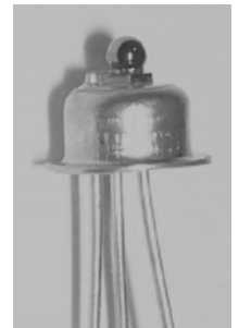
Fig.5 Photo of a ~1 mm wide chalcogenide glass lens (black ball in the photo) formed by a melting process onto a LED chip mounted onto a TO-18 header
