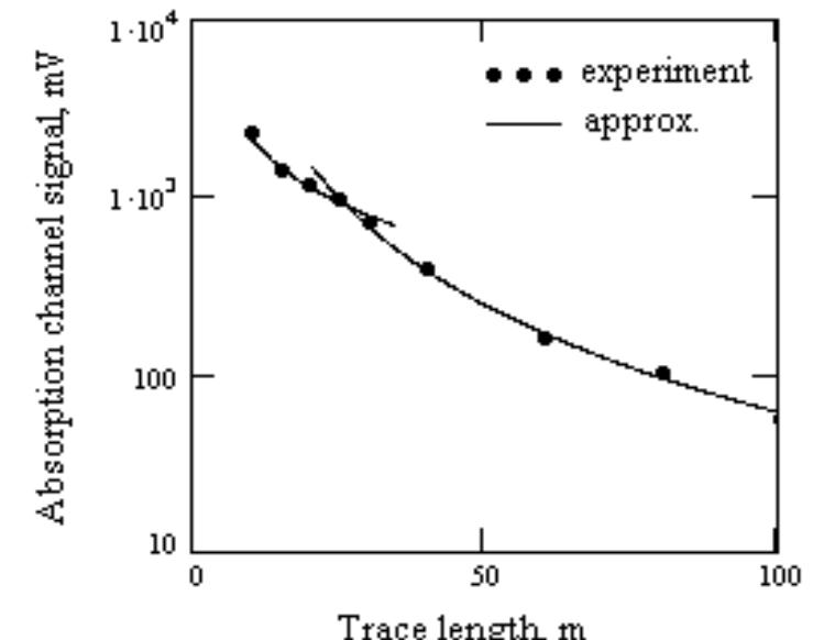
Fig.2. Absorption channel signal vs trace length.
