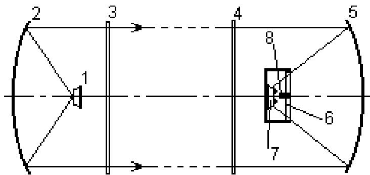
Fig.1. The optical scheme of a trace gas analyzer:
