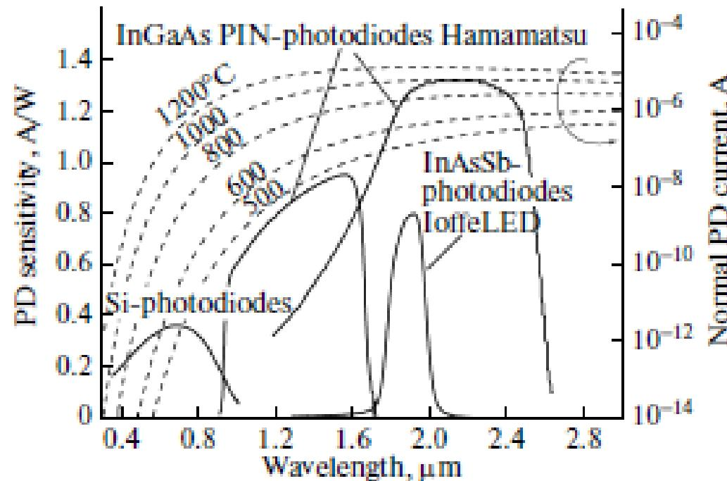
**Fig. 1.** Spectral sensitivity ranges of photodiodes (PD), satisfying the requirements to the developed pyrometric sensor (solid curve), and the "conditional" photodiode currents ( $S = 1 \text{ A/W}$ ) for various spectral regions when detecting 10% of the thermal radiation of the object (blackbody).
