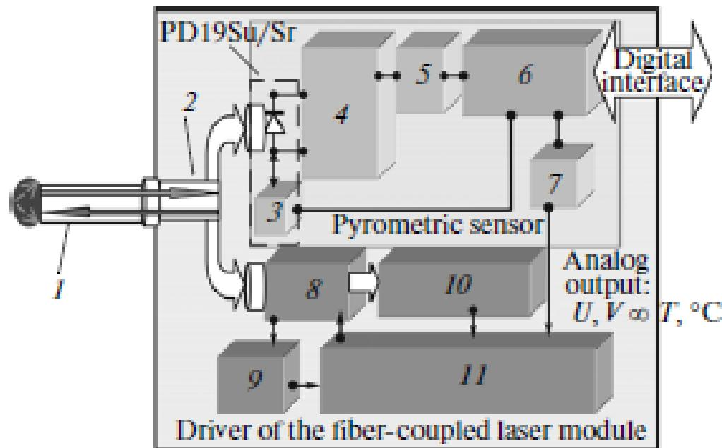
**Fig. 2.** Block diagram of the fiber-coupled laser module driver with embedded pyrometric sensor: (1) operating fiber, (2) Y-shaped fiber splitter, (3) thermoelectric module (TEM), (4) current–voltage amplifier–converter, (5) ADC, (6) control and processing unit, (7) DAC, (8) laser diode, (9) current sensor, (10) radiation–power sensor, and (11) controllable source of stabilized laser pump current.
