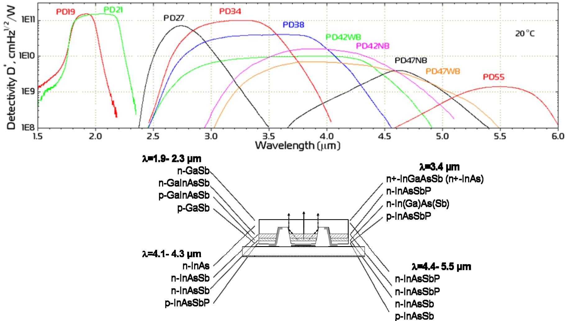
All developed **InAs** and **GaSb** based heterostructures enable flip-chip assembling technology and mounting of an immersion lens on top of the broad band “window” surface (Patent numbers 2261501, 2286618 )
