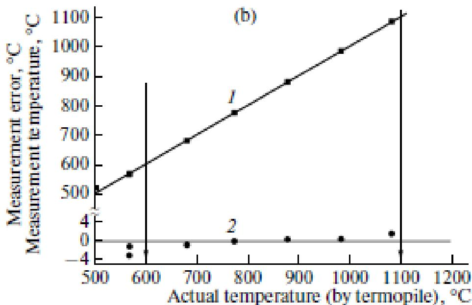
Fig. 3. (a) Experimental PD currents (squares  $I$ ), calculated transfer function of the pyrometric sensor (solid line  $J$ ), experimental (circles  $\Delta$ ) and calculated (dashed line  $\Delta$ ) instrumental errors of the pyrometric sensor. (b) PD sensor readings ( $J$ ) when measuring the temperature at the fiber tip in contact with the emitter and their deviations ( $\Delta$ ) from the emitter temperature measured by a thermocouple.
