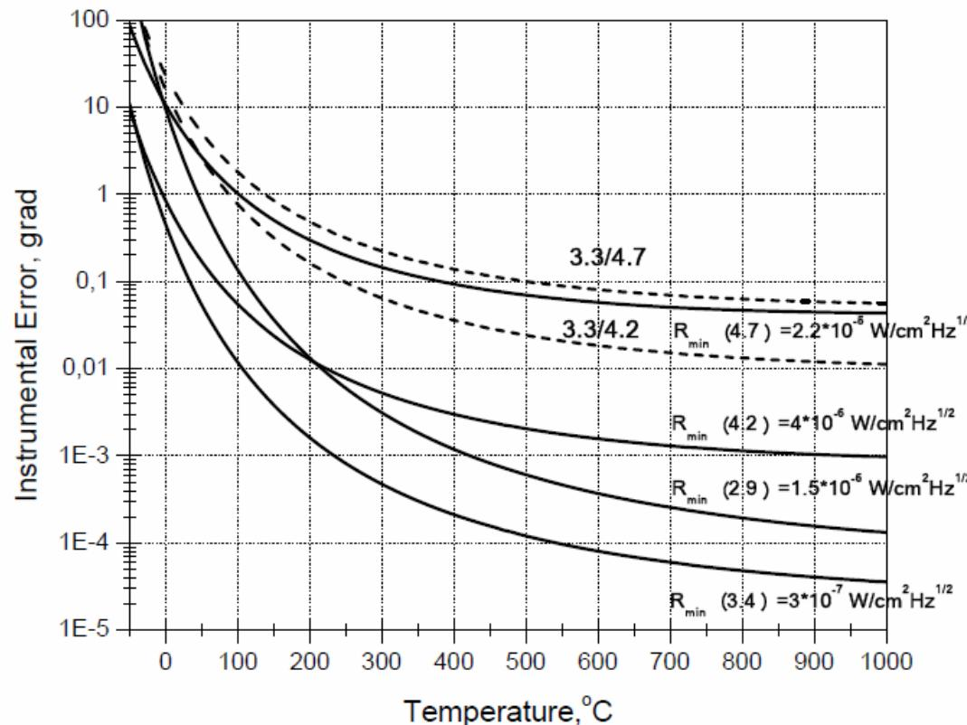
Figure3. Instrumental errors of one-color pyrometric sensors based on A3B5 photodiodes (solid lines) and two-color pyrometric sensors based on pairs of diodes (dotted lines). The time of measurement is equal to 1 s, the linear sizes of the object under measurement are equal to 1 cm, the sighting coefficient is equal to 1:100, the product  $\varepsilon(\lambda)\tau(\lambda)=1$ .
